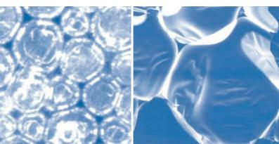
The principle of stability, copied from nature: the linked honeycomb structure of KAPA® polyurethane hard foam core seen under a microscope.
