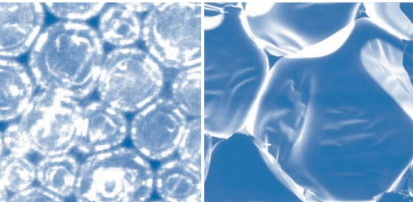
The principle of stability, copied from nature: the linked honeycomb structure of KAPA® polyurethane hard foam core seen under a microscope.
